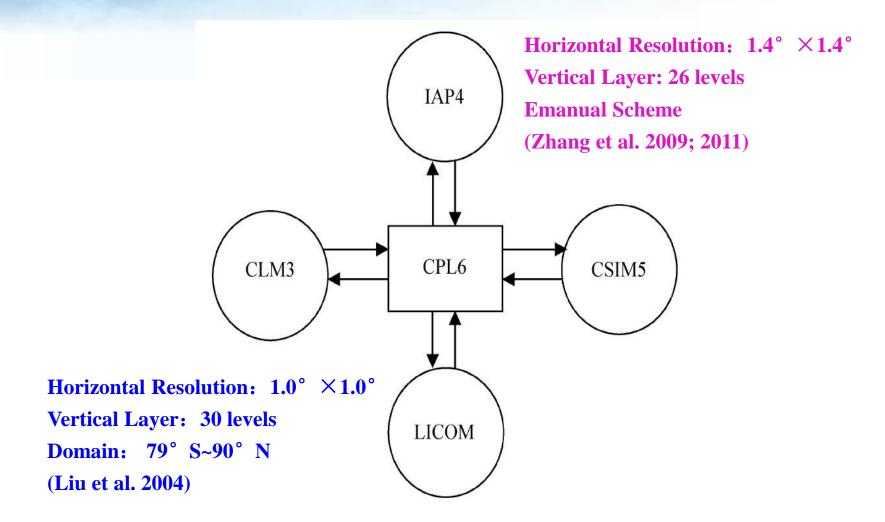
fully coupled climate system model developed by Institute of Atmospheric Physics (IAP)
